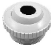
Inlet Fitting 1-1/2" Thd 30220 Inlet: 3/4" Opening 30225 Inlet: 1" Opening 30216 Inlet: 1/2" Opening 30219 Inlet: Slatel Opening
